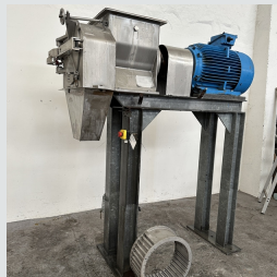
Broyeur râpe inox 22 KW S/S grater grinder
