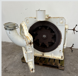
Broyeur centrifuge 110 KW TECHNOPOUDRE type TPB 700 Steel centrifugal grinder
