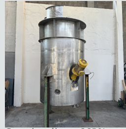
Cuve de mélange 2650L double enveloppe Double jacket mixing tank
