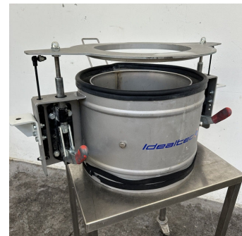
4 systèmes de raccordement de big bag IDEALTEC Big-bag S/S connecting device
