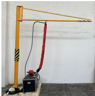
Unité de levage 50 kg Vacuum lift system
