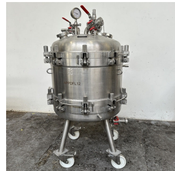
Filtre EUROFILTEC inox Ø 800 mm S/S single plate filter
