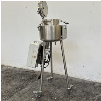
Cuve agitée 7 litres double enveloppe S/S mixing tank dbl. jacket
