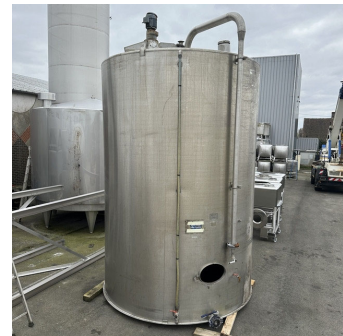
Cuve inox agitée 24m3 PIERRE GUERIN S/S agitated tank
